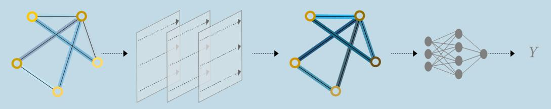
GNN transformations from left to right: input graph  $\rightarrow$  inner architecture  $\rightarrow$  transformed graph  $\rightarrow$ classification processing  $\rightarrow$  output. Visual Credit: Google Research, 2021
